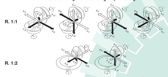
Pinion with left-handed spiral as the drive wheel Sprocket with right-handed spiral as the driven wheel
